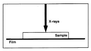
Figure 1.—Conventional film radiographic set-up.
