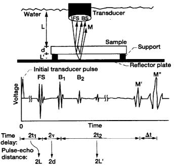
Figure 3.—Single-transducer thickness-independent ultrasonic measurement set-up.
