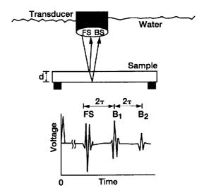
Figure 2.—Conventional pulse-echo ultrasonic measurement set-up.
