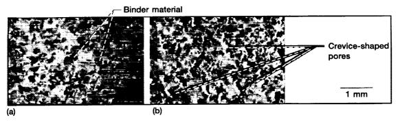
Figure 7.—High density/high velocity and low density/low velocity sections of wheel D10T4.
