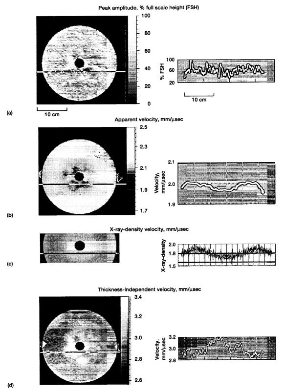
Figure 6.—NDE images and corresponding line profiles at horizontal position near the center of the abrasive cutoff wheel. (a) Conventional pulse-echo ultrasonic c-scan peak amplitude image (B1 gated) and peak amplitude
