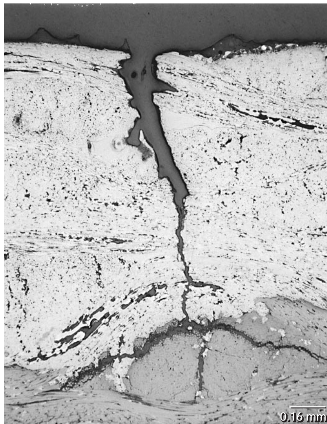
Figure 6.—Continued. (b) Pinhole from OV-102, Wing Leading Edge Panel 12 RH, 15 flights. Cross-sectional view is an optical micrograph.
