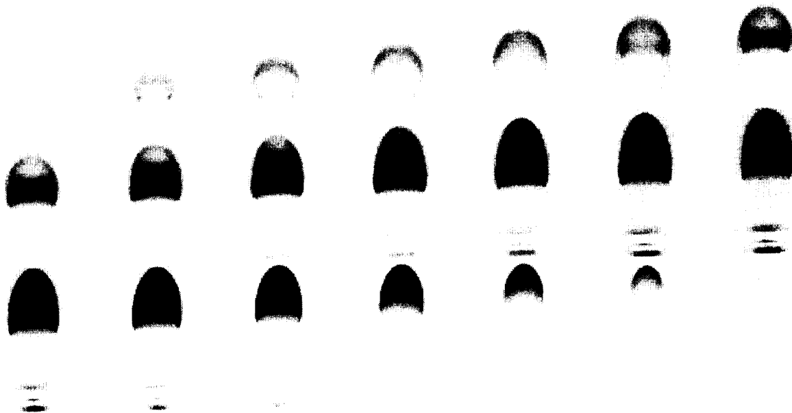
Fig. 3 Flame/vortex interaction using ethane as fuel, V = 26 cc and \Gamma = 282 cm 2 /sec. The observed burnout time is 633 msec. Compare to Figs. 1 & 4.
