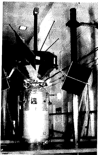
Explorer XIV, launched in October 1962, was designed to investigate solar wind and radiation phenomena.
