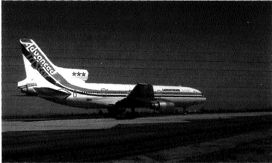
Lockheed L-1011, showing its rear engine installation. (Lockheed)
