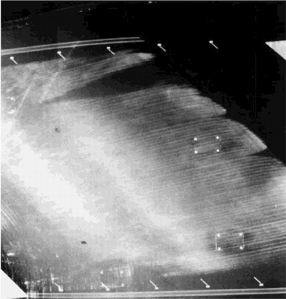
Figure 44. Naphthalene flow visualization at \alpha = -4^\circ and R_c = 1.93 \times 10^6 .
