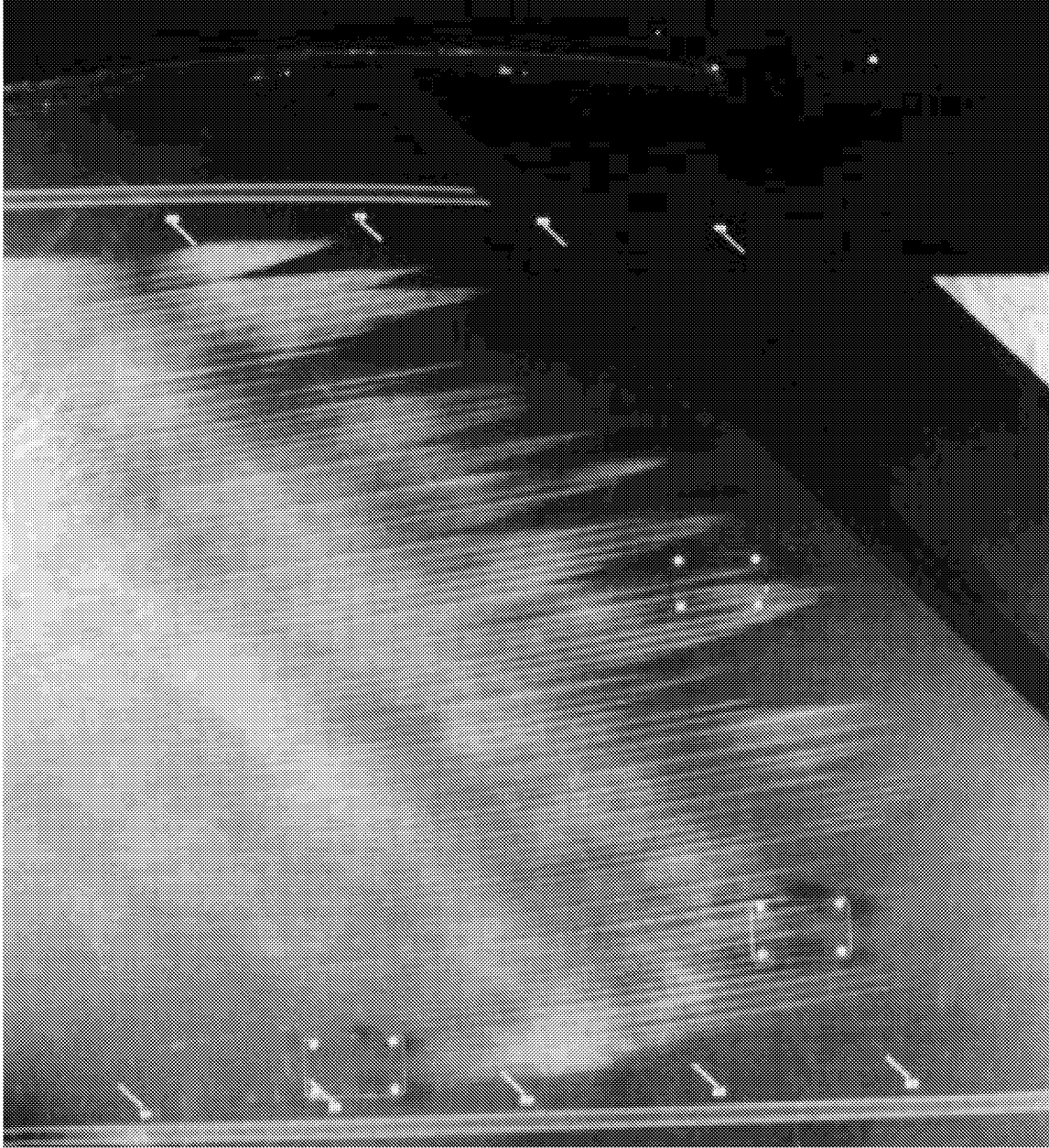
Figure 45. Naphthalene flow visualization at \alpha = -4^\circ and R_c = 2.19 \times 10^6 .
