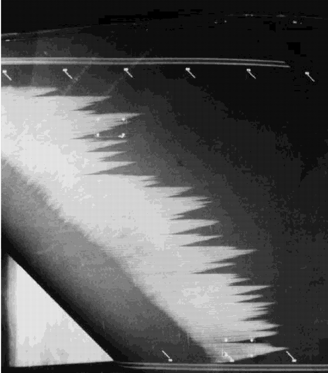
Figure 48. Naphthalene flow visualization at \alpha = -4^\circ and R_c = 3.27 \times 10^6 .
