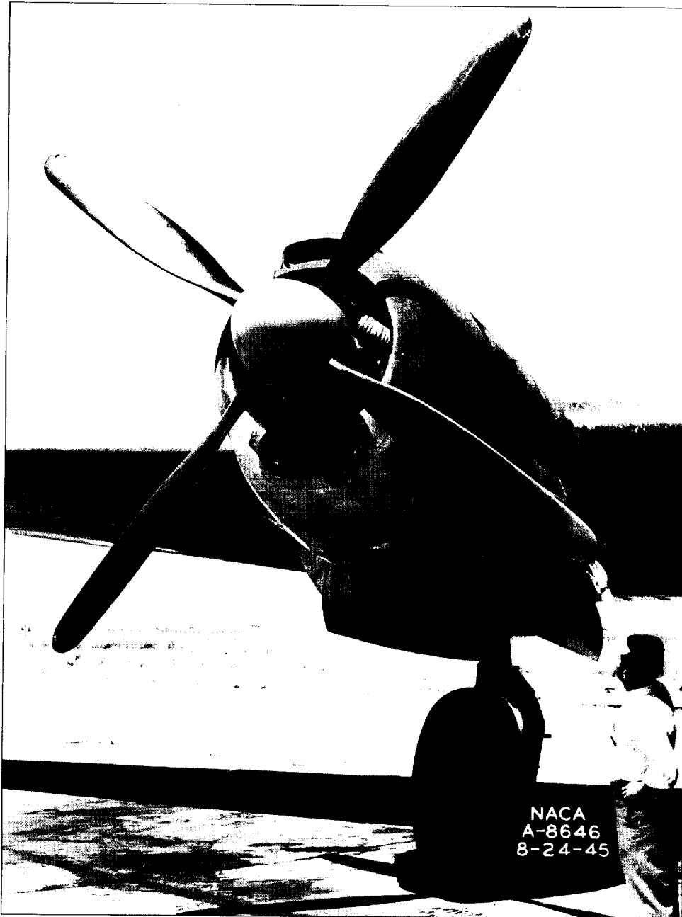
An air-heated propeller designed by Curtiss and installed on the NACA C-46. The heated air exhausted out the orifice at the tip of each blade. (NASA photo no. Ames A-8646).
