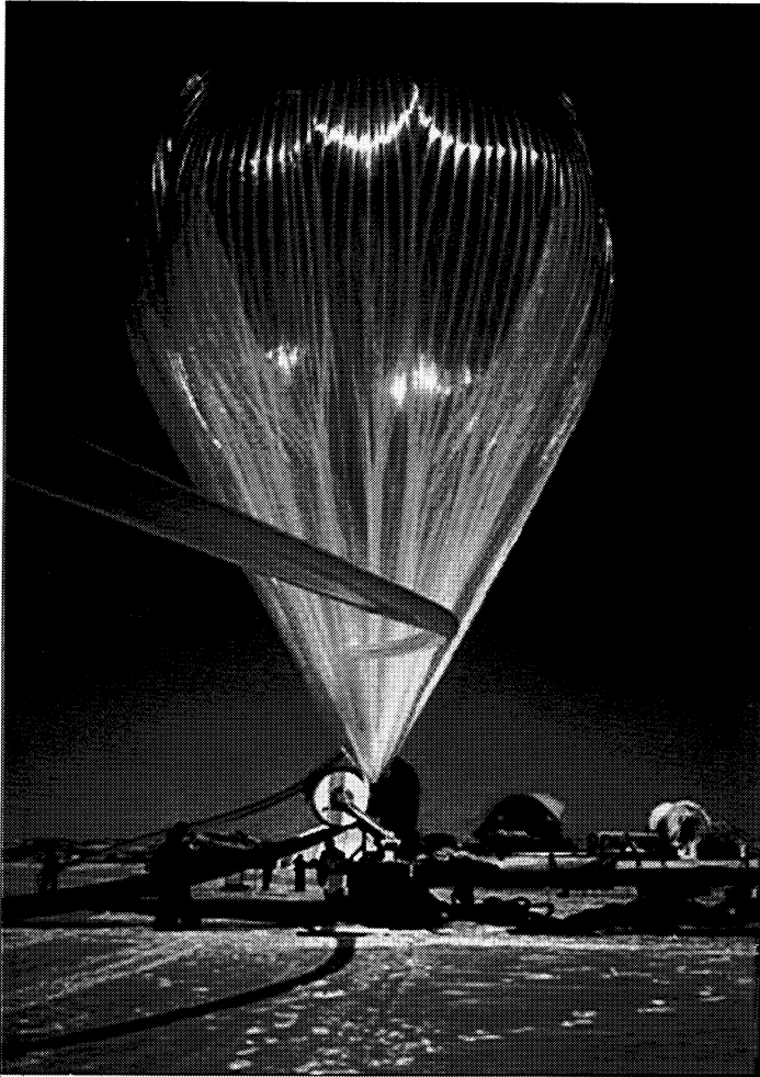
A 30-million-cubic-foot helium balloon (above) which will carry a cosmic ray detector (below) into the stratosphere is prepared for launch in the Antarctic.
