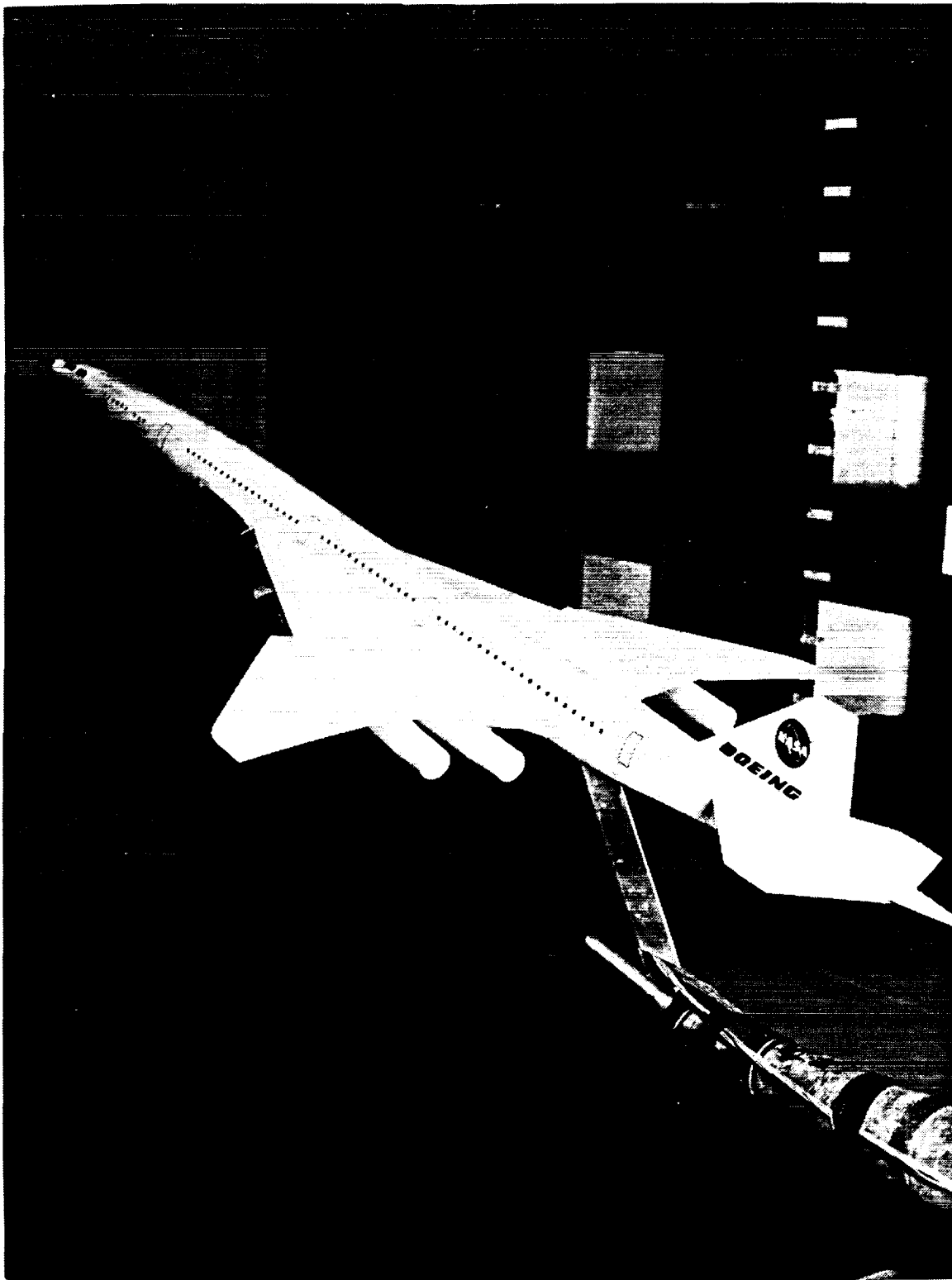
Figure 1. 6% Ref H model shown mounted in the 14- by 22-Foot Subsonic Tunnel..
