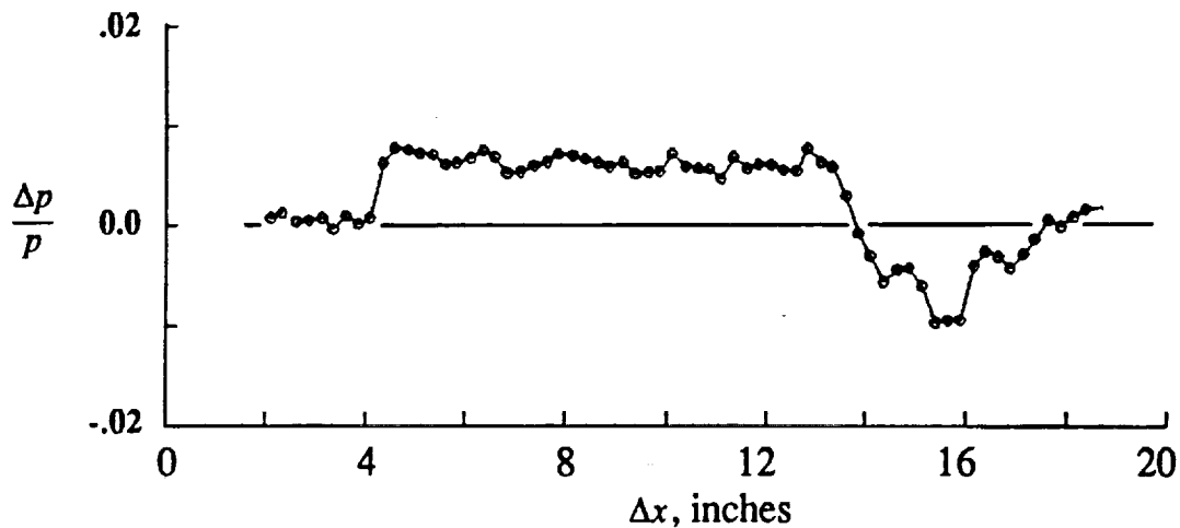
Figure 4. Initial pressure signature from the HSCT-10B model with small nacelles at M = 1.8 , h = 24 inches, and C_L = 0.0519 .
