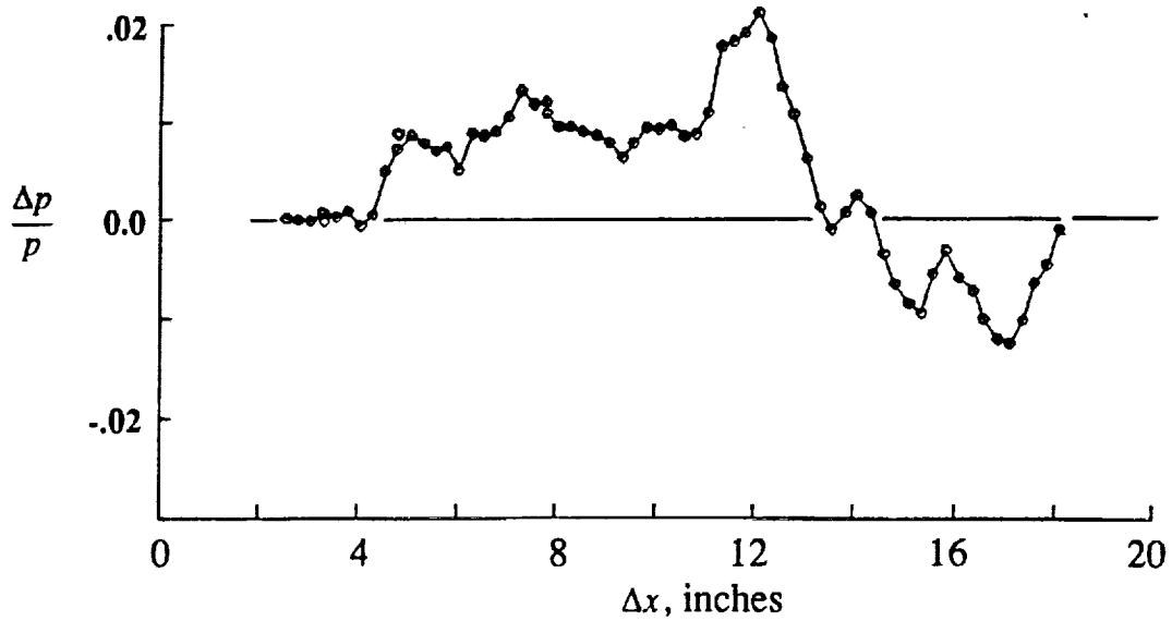
Figure 5. Pressure signature of the HSCT-10B model with small nacelles at M = 1.8 , h = 24 inches, and C_L = 0.1022 .
