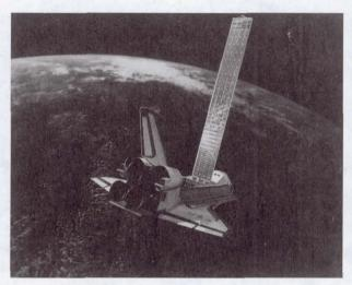
Advanced technology solar array tested in space.
