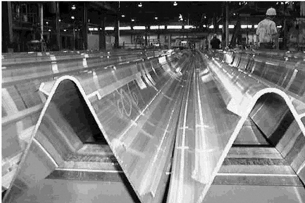
FIGURE 3-12. EXTRUSION CUT INTO LENGTHS
