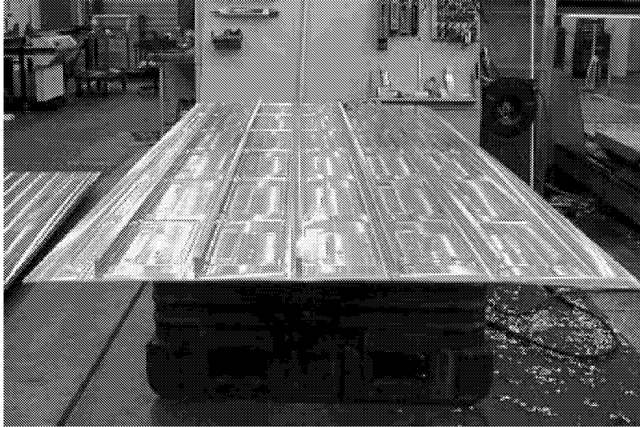
FIGURE 3-3. LOWER PANEL OF TWO-BAY LONGITUDINAL CRACK PANEL AFTER MACHINING
