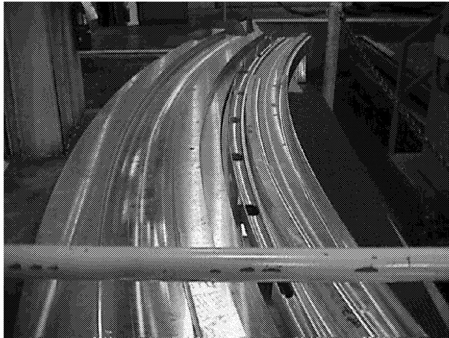
FIGURE 3-6. ROUGH STOCK AND MACHINED FRAME
