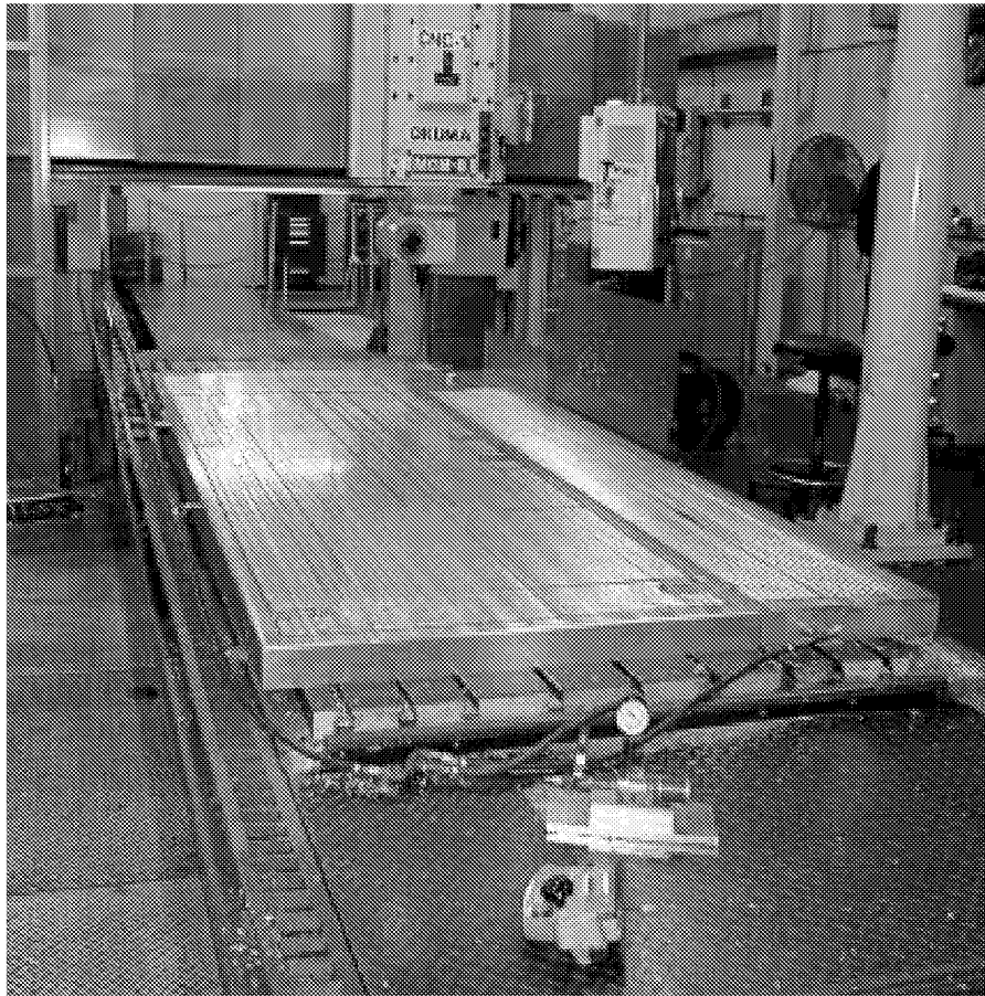
FIGURE 3-1. THREE-AXIS, FIVE-FACING, 3000-RPM MILLING MACHINE
