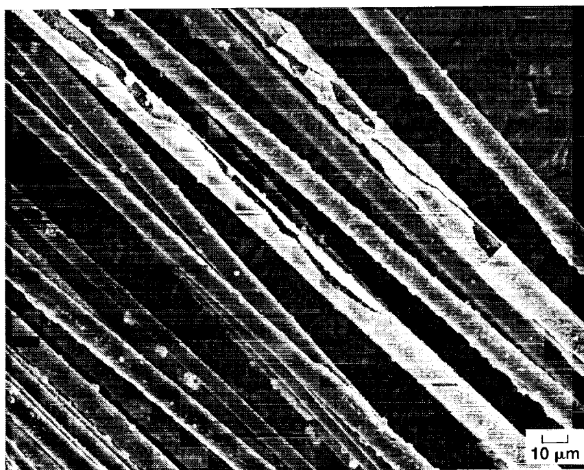
Figure 10.—SEM micrograph from surface of monazite-coated Sylramic fiber.
