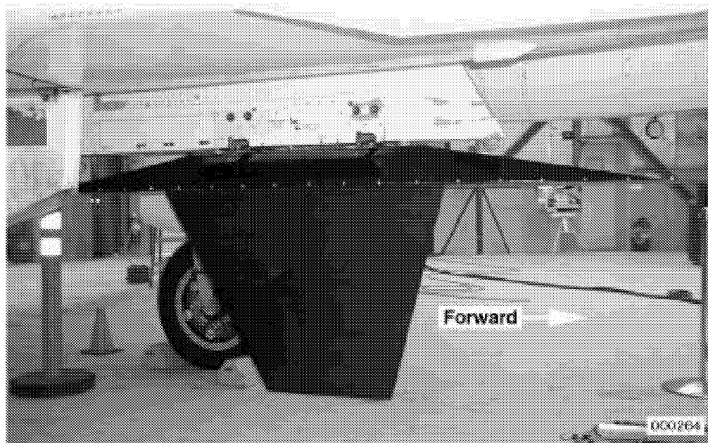
Fig. 3. Supersonic natural laminar flow test article mounted on NASA F-15B aircraft.
