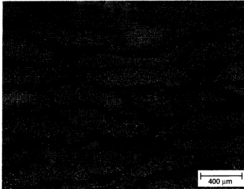
Figure 1.—Optical micrograph of the cross-section of a 1-D BN/SiC coated Hi-Nicalon SiC/RBSN composite ( V_f \sim 0.24 ) showing infiltration of silicon nitride matrix between the filaments within the fiber tows, and matrix rich regions between the fiber tows.
