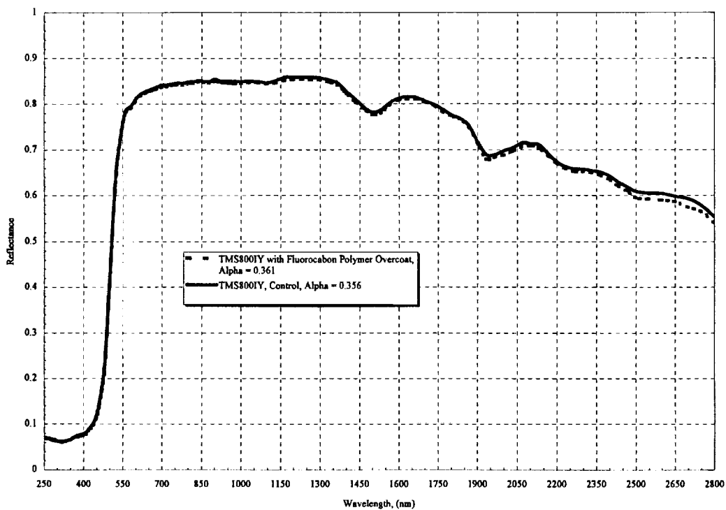
Figure A-8. TMS800-IY Handrail Witness Panel with Fluorocarbon Polymer Overcoat
