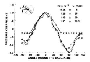
Fig. 3 Pressure distributions on a cricket ball held at a seam angle of 20°.
