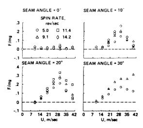
Fig. 4 Variation with flowspeed of the normalized side force (averaged over 5 balls).
