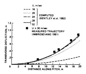
Fig. 5 Computed flight paths using measured forces for the cricket ball with the best swing properties. Seam angle =  $20^\circ$ , spin rate = 14 revs/sec.
