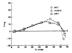
Fig. 8 Effect of humidity on the measured side forces on a spinning cricket ball. Seam angle = 20°, spin rate = 5 revs/sec.
