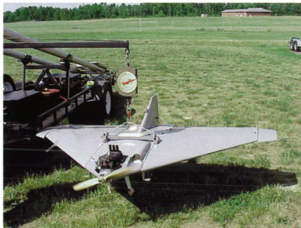
An Exdrone undergoes weight and balance tests.
