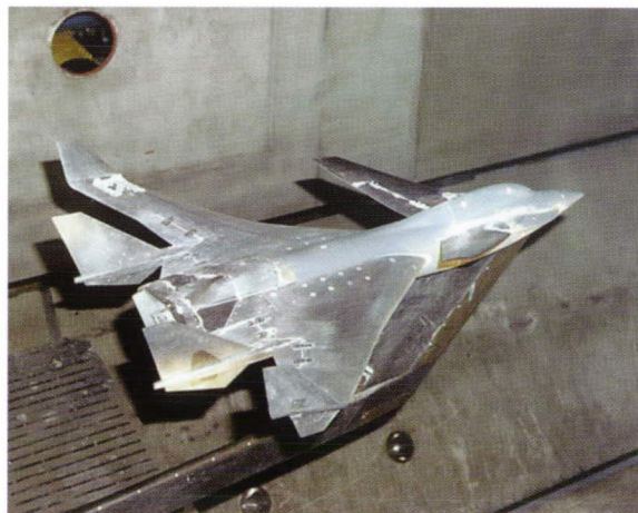
The original HiMAT model with the thrust-vectoring, wedge nozzle in the Langley 16-Foot Tunnel.
