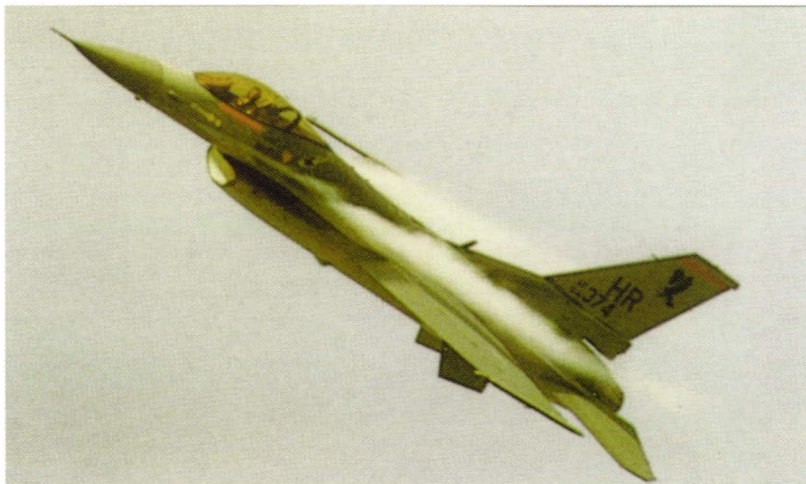
F-16 in a hard turn with wing leading-edge flaps deflected and vortices produced by the sharp wing-body strakes illustrated by condensation.
