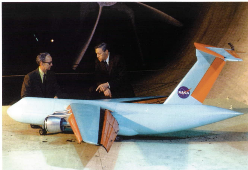
Langley researcher John P. Campbell (l) and Gerald G. Kayten (r) of NASA Headquarters inspect a free-flight model of an EBF configuration in the Langley Full-Scale Tunnel.
