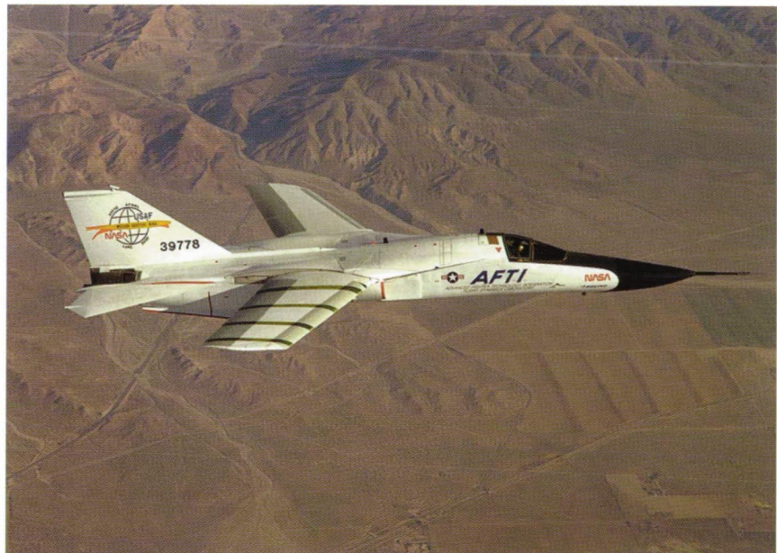
The F-111 Mission Adaptive Wing (MAW) aircraft during flight tests at Dryden.
