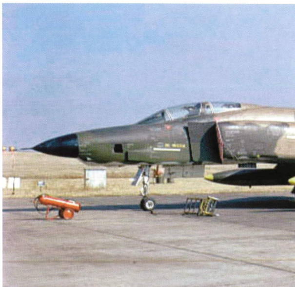
The RF-4 reconnaissance version of the F-4 with camera fairing under the forward nose section.
