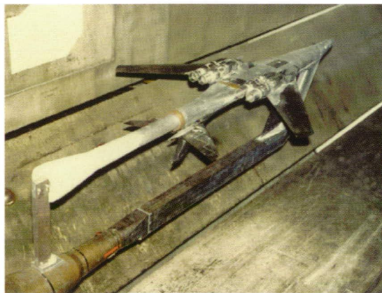
B-1B model in an inverted position for nozzle flap load investigation in the Langley 16-Foot Transonic Tunnel.
