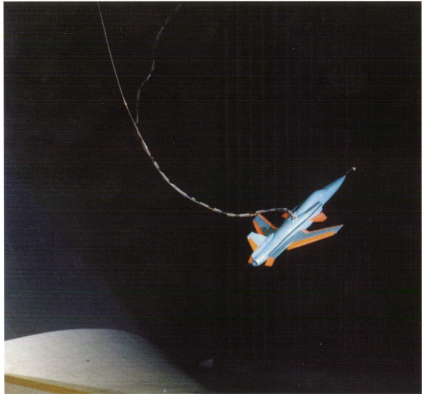
X-29 free-flight model undergoing tests at high angles of attack in the Langley Full-Scale Tunnel.
