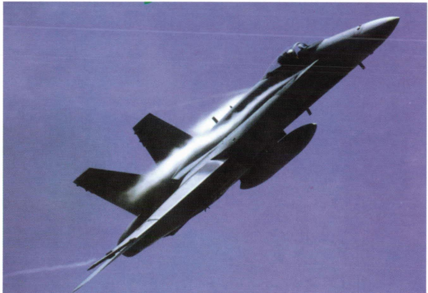
F/A-18 with wing leading-edge flaps deflected and LEX vortices made visible by condensation.
