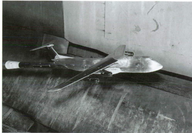
C-5 model mounted for tunnel test section study in the Langley 16-Foot Transonic Tunnel.
