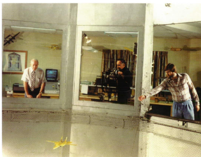
F-14 model in spin recovery tests in the Langley Spin Tunnel.
