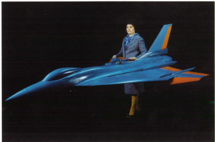
Project engineer Sue B. Grafton with the free-flight model of the F-16XL.
