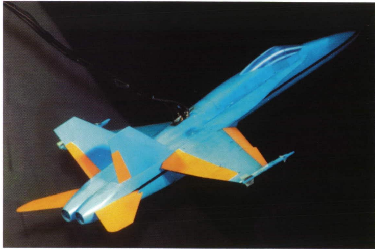
The F/A-18A free-flight model during tests in the Langley 30- by 60-Foot Wind Tunnel in 1978.
