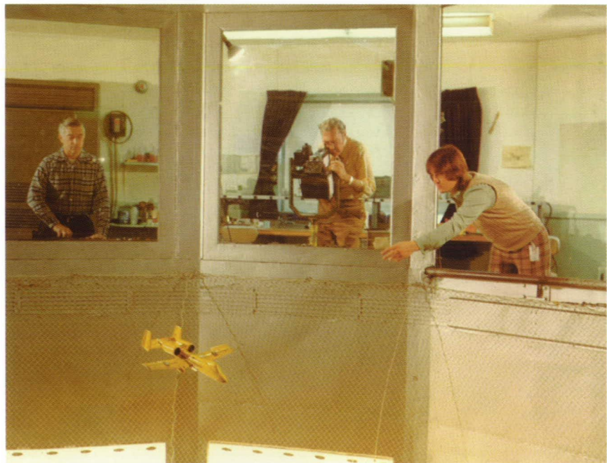
Spin tunnel tests of the A-10 configuration.
