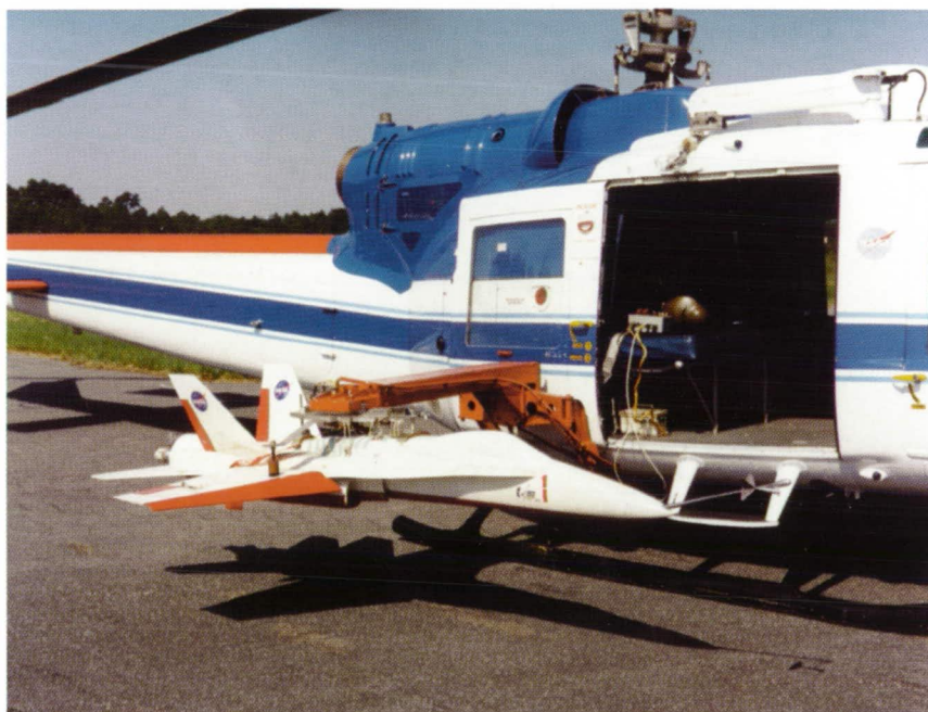
F/A-18 drop model prepared for flight in 1978.
