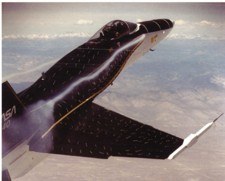
F-18 HARV during flow visualization studies using smoke ejected at apex of LEX and wool tufts on upper surfaces.
