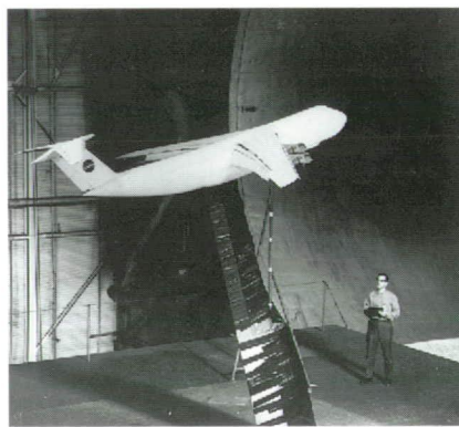
Powered C-5 model mounted in the Langley Full-Scale Tunnel for externally blown flap assessments with the double-slotted flap configuration.
