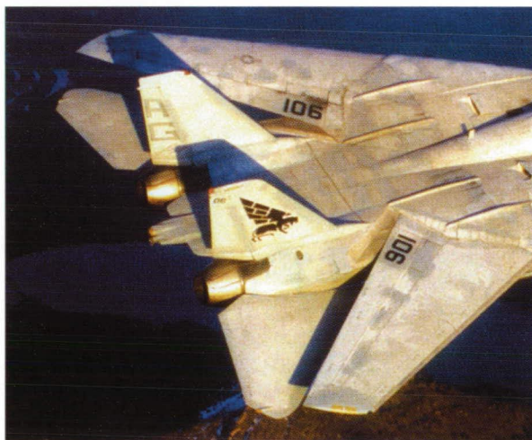
Aft-end pancake handle and vertical tail root speed bumps on F-14 aircraft.
