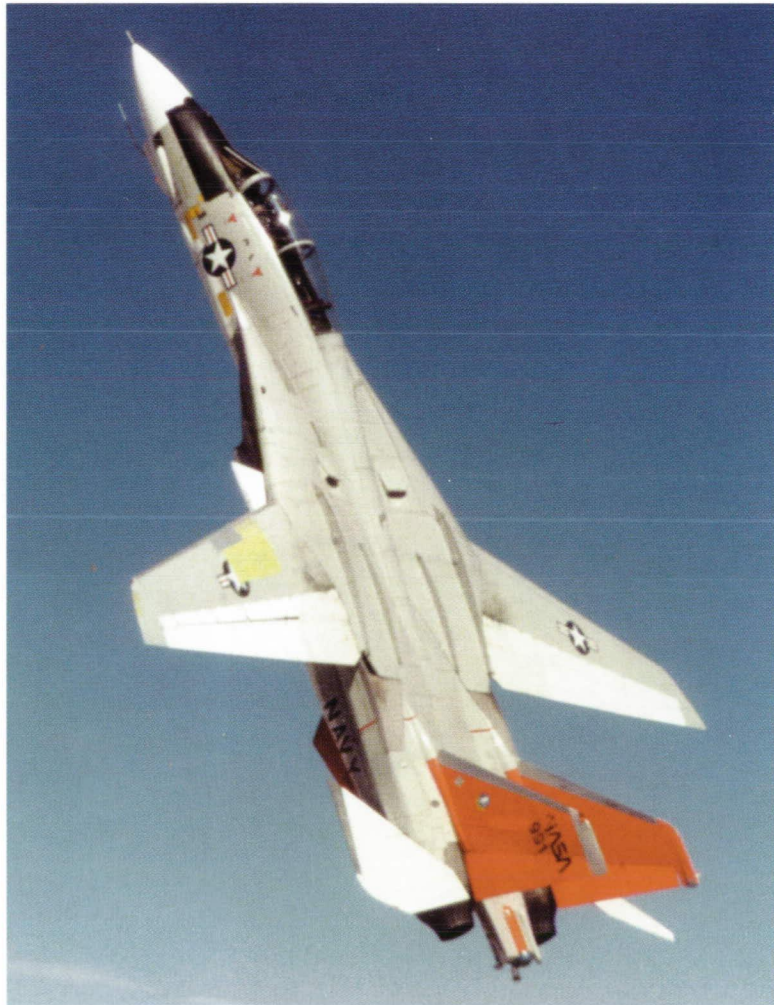
The F-14 responds to an abrupt stick pull by Dryden test pilot Fitz Fulton during evaluations of the Langley designed Automatic Rudder Interconnect (ARI) control system at Dryden.
