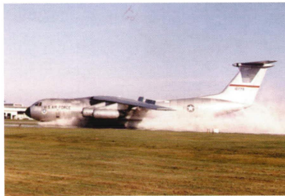
C-141 braking tests in a joint NASA, Air Force, and FAA program at Wallops Flight Facility.
