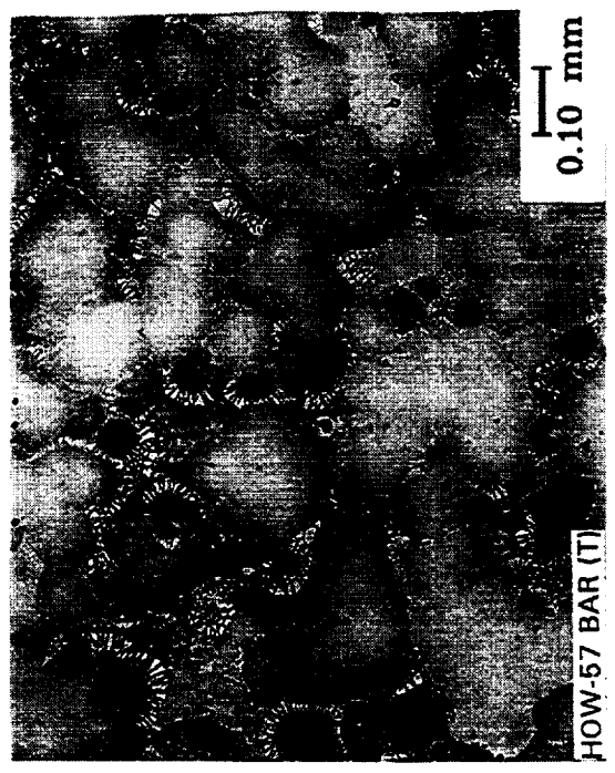
Figure 3. High magnification view of Howmet cast R125 microstructure, a) HOW-16 sheet (T) orientation, b) HOW-16 sheet (L) orientation, c) HOW-57 Bar (T) orientation, and d) HOW-57 bar (L) orientation.
