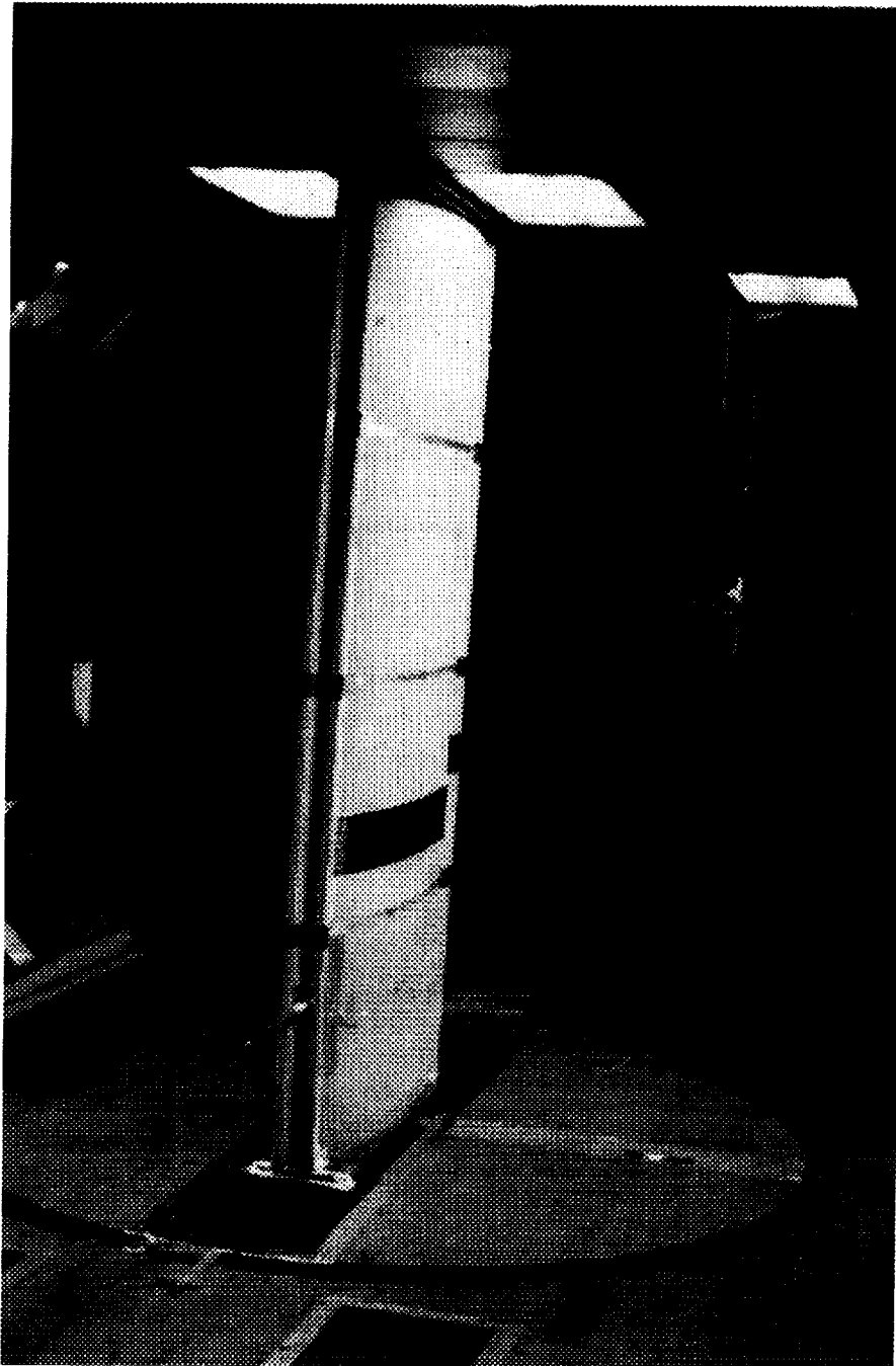
Figure 8 LEWICE Ice Shape Installation (View from Upstream)
