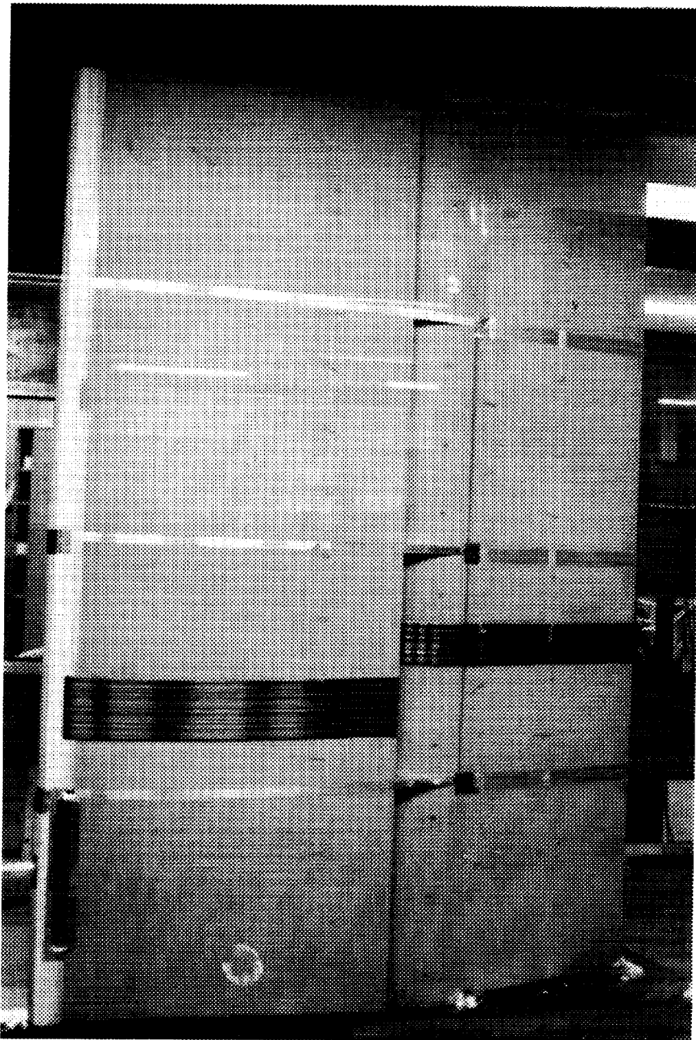
Figure 36 S&C Ice Shape Tuft Flow Visualization, \alpha = -8.0^\circ, \delta_c = 0.0^\circ
