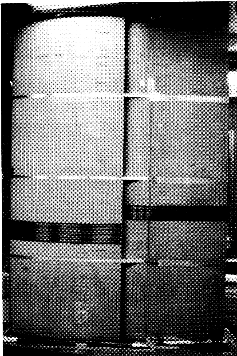
Figure 35 Baseline Tuft Flow Visualization, \alpha = -8.0^\circ , \delta_e = 0.0^\circ
