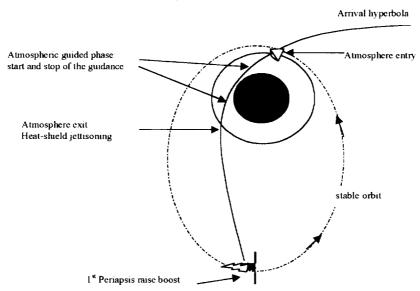
The MSR orbiter will arrive at Mars with an excess velocity of about 3.2 km/s. The objective of the
