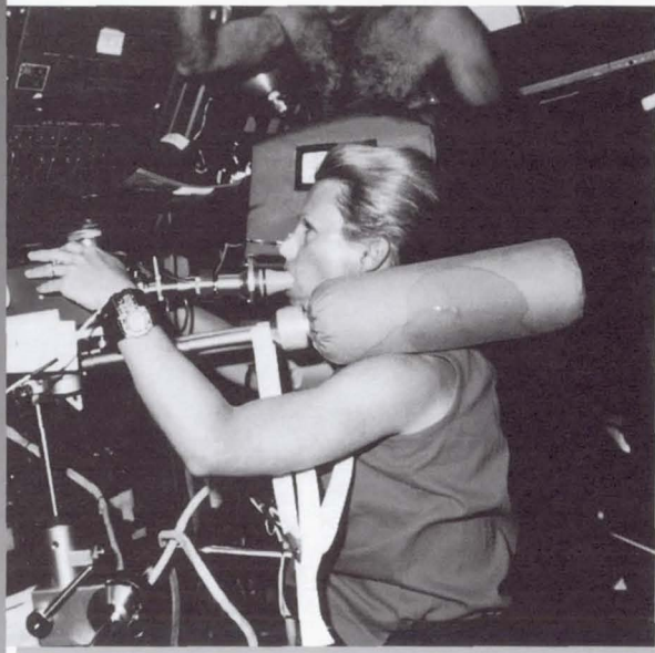
Astronaut Rhea Seddon breathes into the rebreathing unit during the exercise phase of the cardiovascular deconditioning experiment on SLS-2. The results on inflight experiments such as this are applied to alleviate the risk and reduce heart and lung disease on Earth
