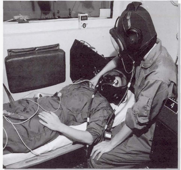
Pre-cordial doppler monitoring in the altitude chamber. Subjects are tested in hypobaric and hyperbaric chambers to assess the risk of decompression sickness using various combinations of cabin pressure, gas composition, and suit pressure.
