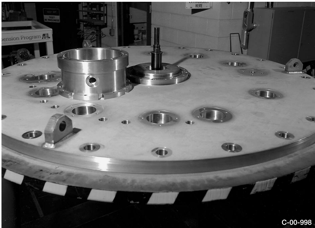
Figure 3.—Top view of rotor without thrust bearing assembly.
