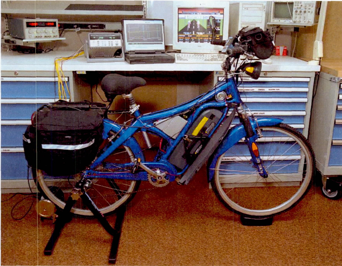
Fig. 2 – EV-Global E-Bike on Dynamometer with Fairing Removed
