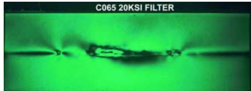
Photostress of Planished Repair Weld
