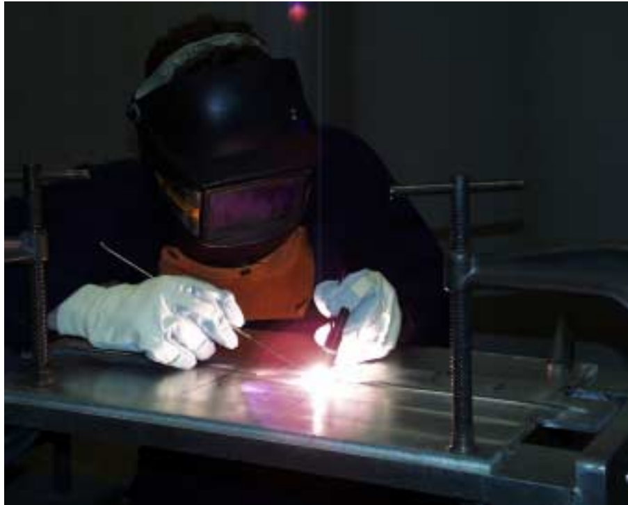
Manual GTA Repair Welding
