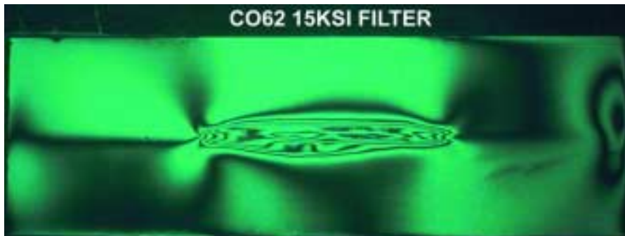
Photostress of Unplanished Repair Weld
