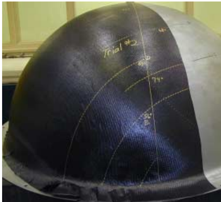
Figure 5: The results of the 5HS cloth drape test on a 36 inch diameter dome. The dashed tracer lines follow individual tows within the cloth. The solid line represents the centerline of the dome.
