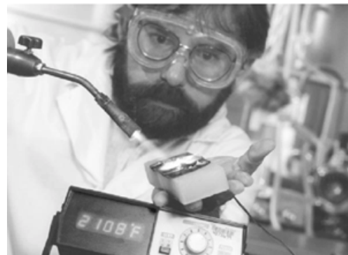
Figure 2: Tom Tillotson, a chemist at Lawrence Livermore, applies a flame to the top of a 1-inch-thick silica aerogel brick. Even though a thermocouple placed on the aerogel's top surface reports a temperature of 2,108°F, his hand is totally unaffected by the heat.
