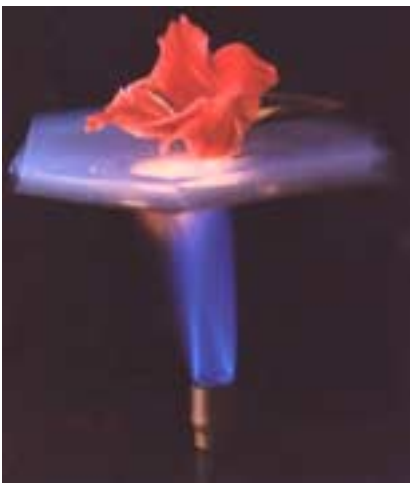
Figure 1: The wispy, fragile appearance of an aerogel shown protecting a flower from being consumed by a burner.
