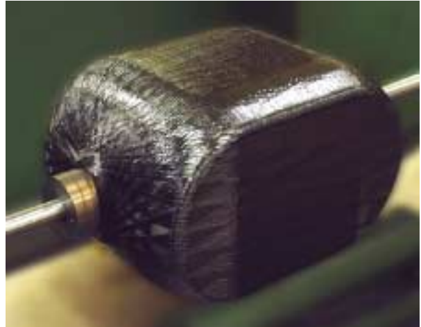
Figure 4b: Helical wound one-fifth scale model of a CBAT Propellant Tank (before cure). Helical winding causes more build up in the domes regions because of the crossovers.
