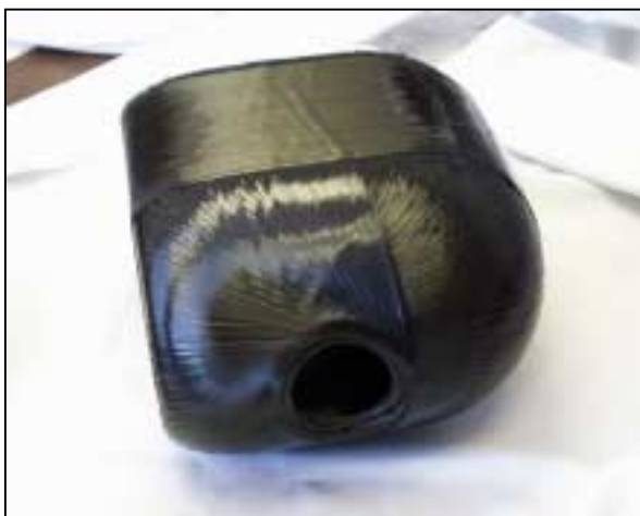
Figure 4a: Polar wound one-fifth scale model of a CBAT Propellant Tank. Polar winding minimizes build up in the domes due to fewer crossovers. The non-cylindrical shape creates fiber tow overlaps in the flat regions.
