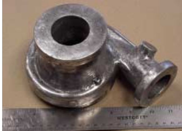
Figure 5. Half-scale Al MMC turbopump housing for X-34's Fastrac Engine.
