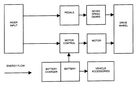
PARALLEL HYBRID SCHEMATIC DIAGRAM
