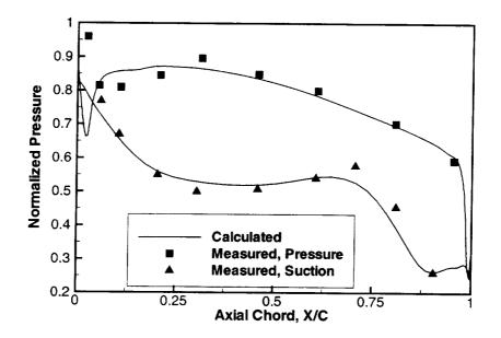
Figure 5. Comparison of steady blade loading for the turbine cascade at an expansion ratio of 2.713
