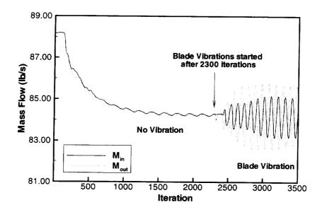
Figure 8. Variation of mass flow for the transonic fan, with and without blade vibration
