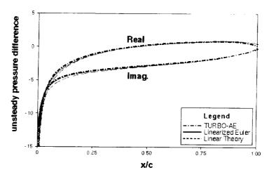
Figure 2. Unsteady pressure difference variation with chord at midspan for 180 deg IBPA plunging oscillations
