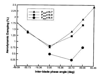
Figure 9. Variation of aerodynamic damping with back pressure and IBPA for the transonic fan with forced blade vibration in the first natural mode at the natural frequency of 351 Hz
