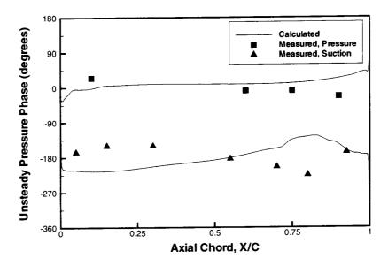
Figure 7. Comparison of unsteady pressure response phase for the turbine cascade vibrating in a torsional mode at 340 Hz, 180° IBPA, and 2.713 expansion ratio
