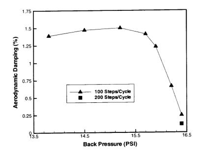
Figure 10. Variation of aerodynamic damping for 16.4 PSI back pressure. Forced vibration in the first natural mode at 351 Hz and 32 deg IBPA
