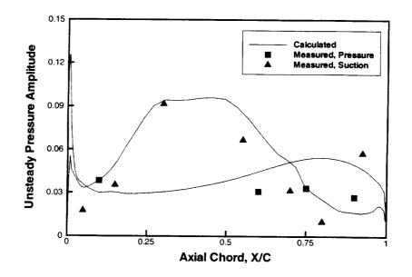
Figure 6. Comparison of unsteady pressure response amplitude for the turbine cascade vibrating in a torsional mode at 340 Hz, 180° IBPA, and 2.713 expansion ratio
