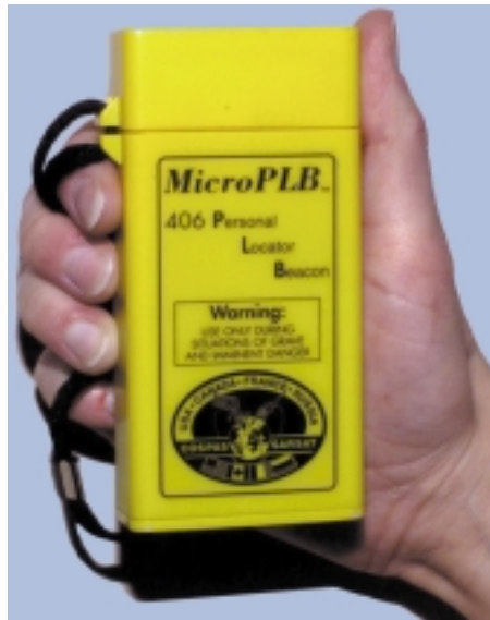
Microwave Monolithic, Inc.'s MicroPLB is a state-of-the-art search and rescue satellite-aided tracking (SARSAT) transmitter.
