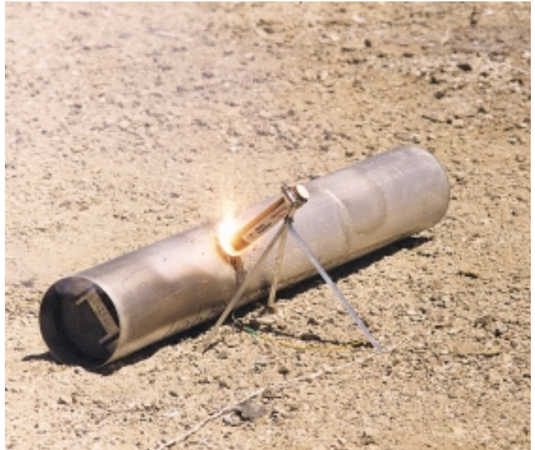
Thiokol Propulsion's demining flare burns through the outer casing to neutralize the explosive agents inside.
