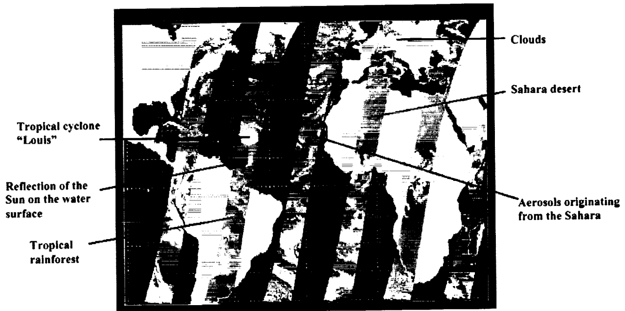
Fig. 3.3 GOME PMD measurements on 2 September 1995 with a 20 \times 40 \text{ km}^2 resolution. OMI will be able to retrieve clouds and aerosols with a similar resolution, but with daily global coverage. (Figure with courtesy of R. Koelemeijer, KNMI)
