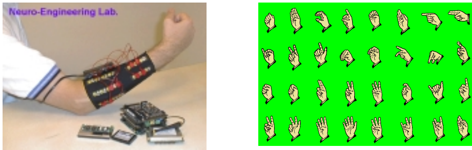
Figure 2: EMG arm band and typical gestures
