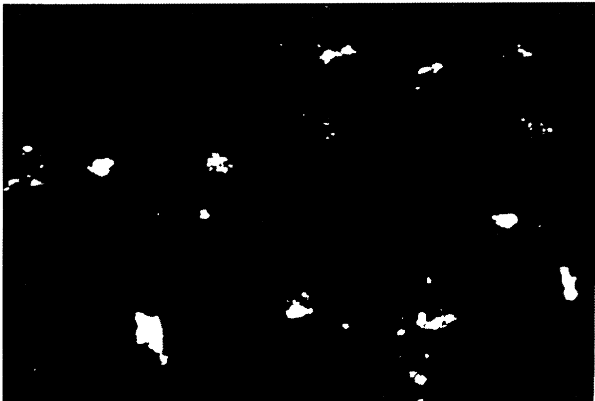
Figure 56: Optical microscopy picture of a 6% (mol) Zr(acac)_4/PI film (top:brightfield, bottom:darkfield)
