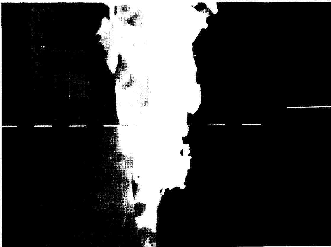
Figure 40. Flake on a crack of a 8% (mol) Zr(acac)_4/PI film at 80x and 30° tilt
