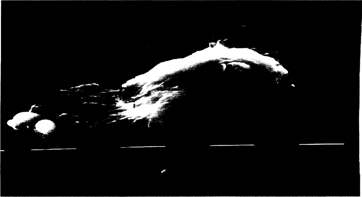
Figure 42a. Feature in a 10% (mol) Zr(acac)_4/PI film at 1250x 35° tilt
