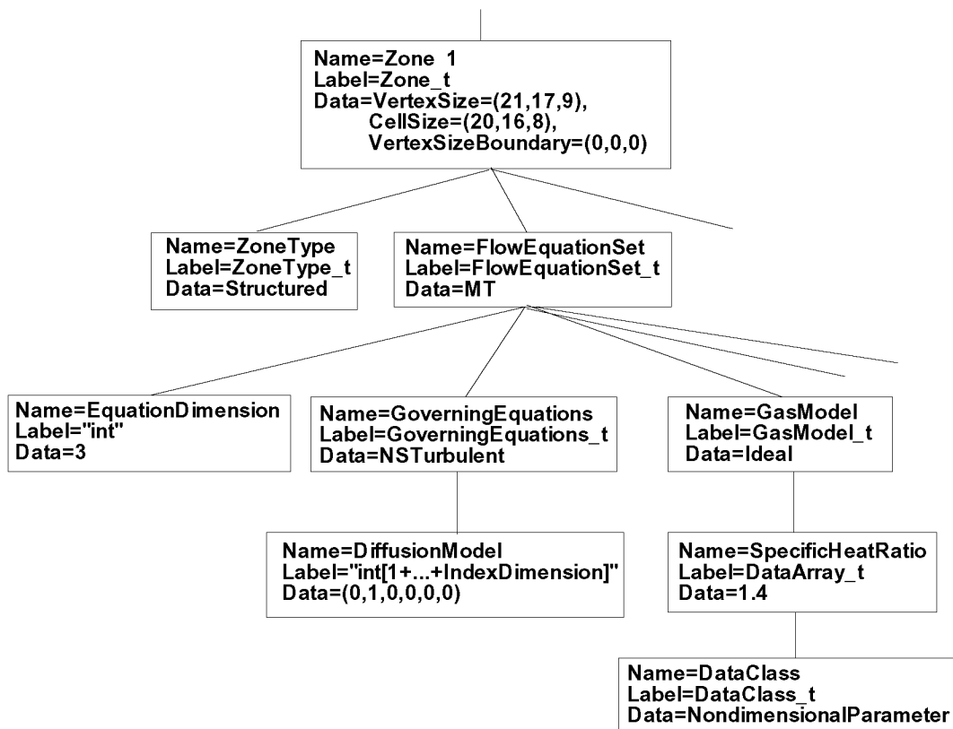
Figure 19: Layout of part of a CGNS file with flow equation set information.
