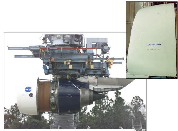
Figure 9. Boeing scarf inlet installed on a Pratt & Whitney PW4098 engine. Photo reproduced from Ref. 6.
