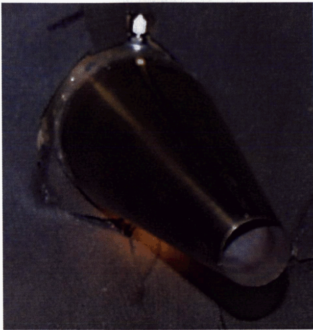
a) 1.60-inch diameter convergent round nozzle
