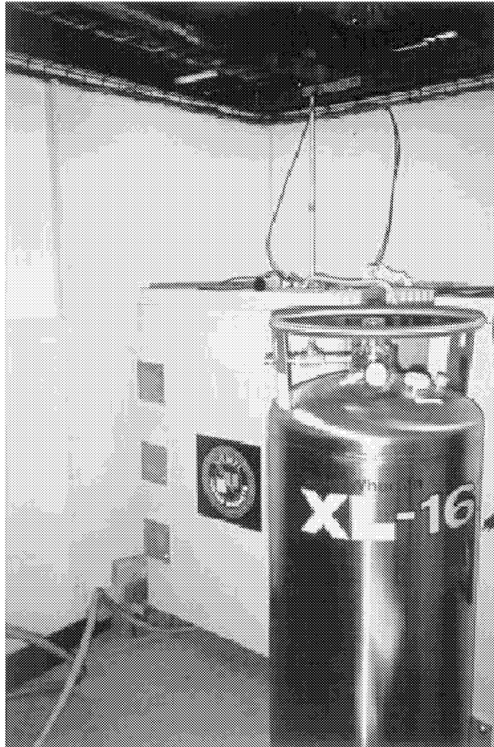
Figure 15. Sealed test article container prior to a pulsed test at the NHMFL Los Alamos facility.
