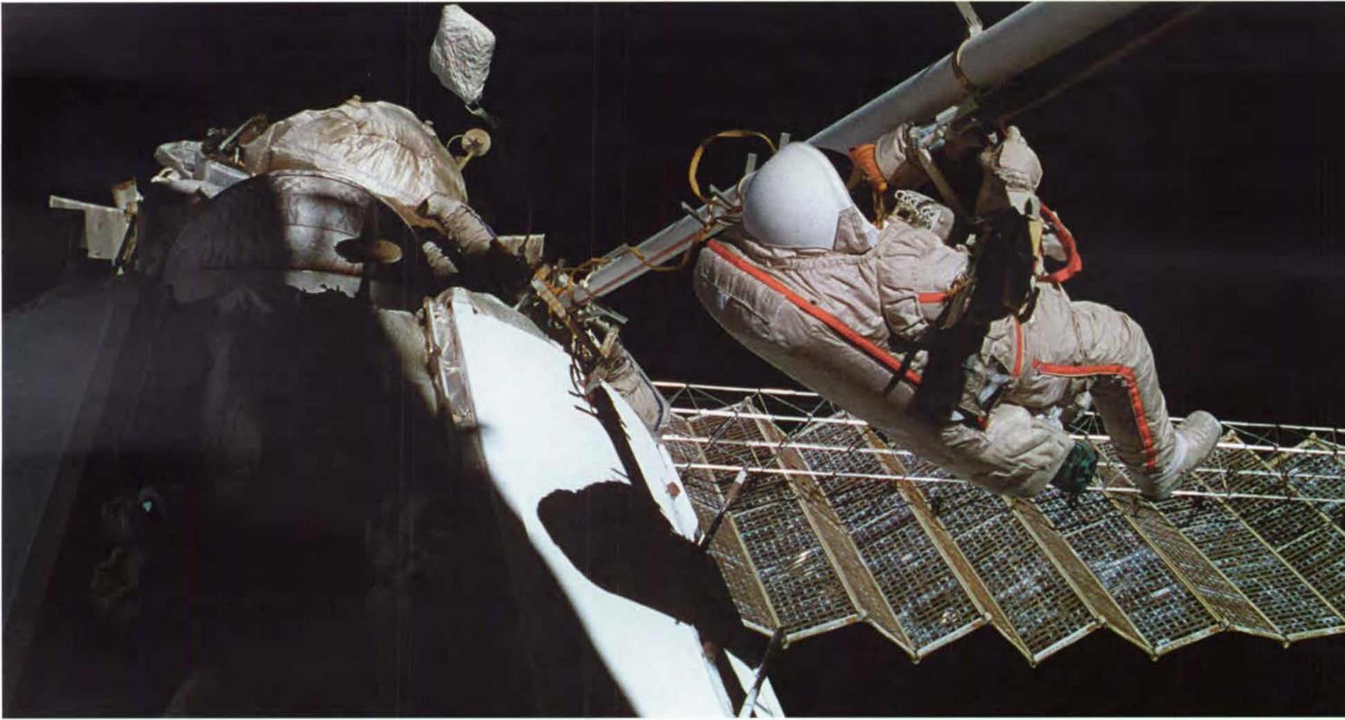
Commander Dezhurov (above) works outside the Mir space station to fold and move a set of solar arrays. Red stripes on the Russian Orlan extravehicular activity suit mark his rank as the commander.
