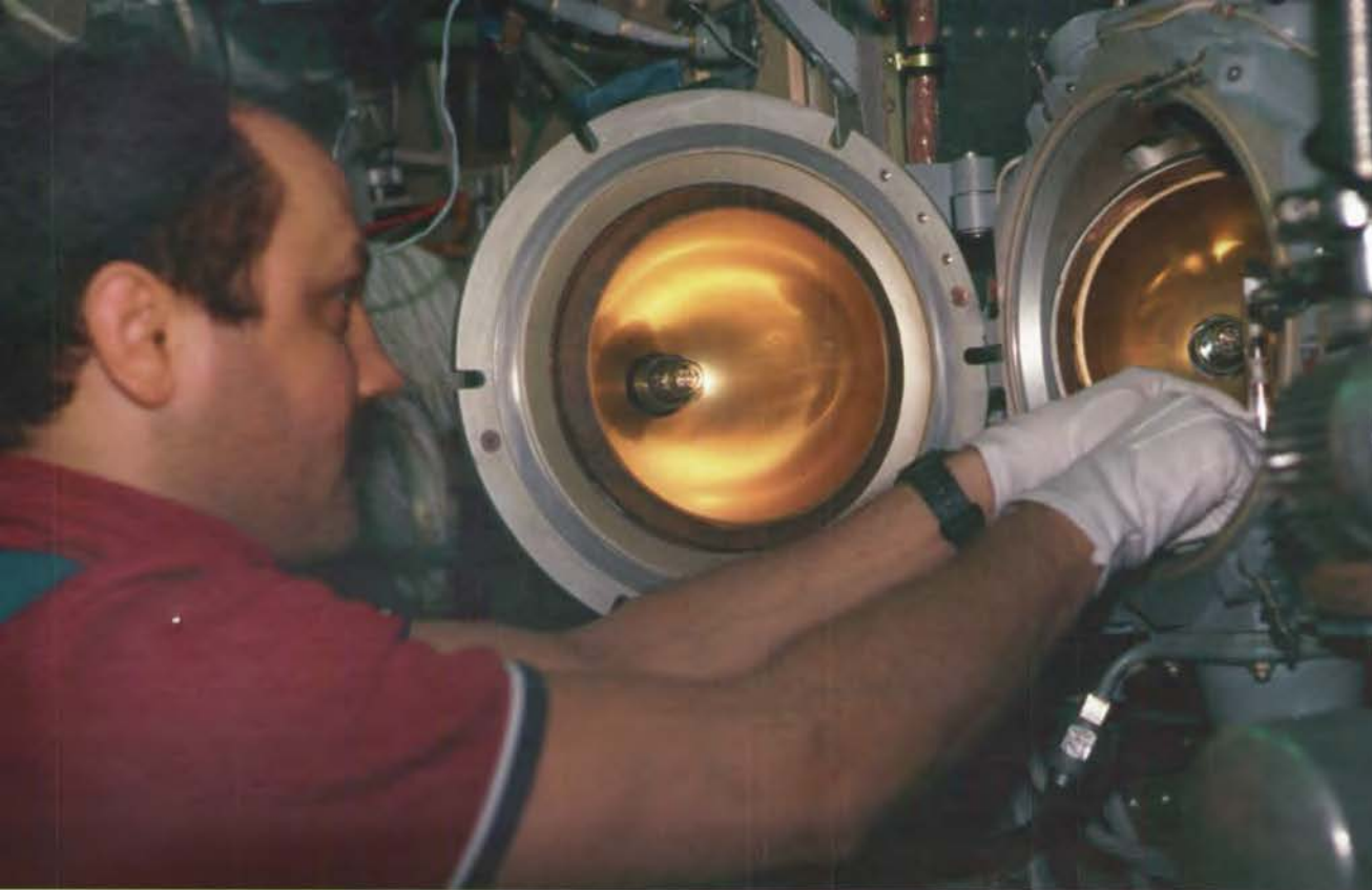
Mir-21 Commander Onufriyenko (photo left) and Flight Engineer Usachev (in suit with blue stripes) traverse an existing truss on the Kvant module during one of their six spacewalks. (Above) Usachev inserts metal samples into the QUELD furnace. (Below) Lucid chooses reading material from the Mir library located in the Spektr.
