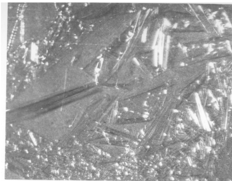
Figure 11: Micrograph of sample ssa-05 showing increased severity of coating spalling following VUV exposure as evidenced by coating flaking off of entire sample.
