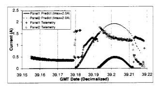
On February 17, 2001 (GMT 48), one of the only Xpop periods of FPP housekeeping data was obtained. This had the STS present, an Xpop flight mode with a YPR of (0,-6,0) degrees, gimbals locked and a solar beta angle of about -5 degrees. It was not possible to deduce the Imax
