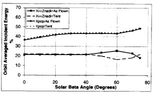
The following figure shows the orbit averaged incident energy for the two flight modes over the entire solar beta angle range.
