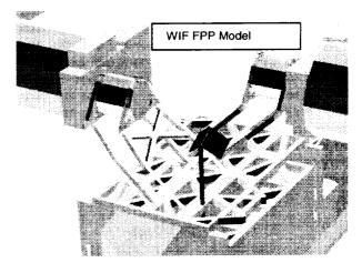
The final FPP as-flown design implemented the recommended solar panel configuration in a different appearing yet energy equivalent way. A geometry model of this version was created, including hexagonal body, probes, antenna,
