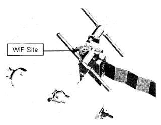
At this time in the design process, it became clear that the optimum orientation of the solar arrays did not match the original tent configuration. Models for several different orientations were considered, with the ultimate configuration of the solar panels being a tent (as before) rotated about the Z axis by 90 degrees and canted aftward about the Y axis by 30 degrees.
