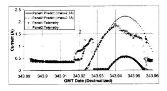
The next comparison occurred when the FPP resumed operation on January 29, 2001 (GMT 29). The STS was not present, a XvvZnadir flight mode with a YPR of (0,-8,0) degrees, gimbals locked and the solar beta angle was about 30 degrees. The conditions were similar to the December data, and seemed to match the predictions.
