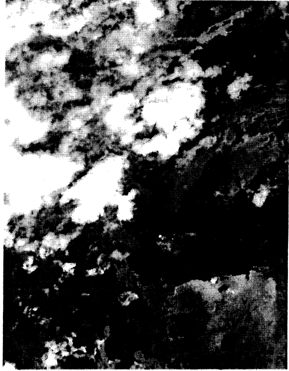
Figure 5. AVIRIS image at 1503.4 nm showing mixture of solar reflected radiance and hot target radiance from the active volcanic vent.
