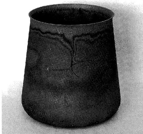
Figure 11 – Post-test image of CR-side RZL (555-07-005). Note the oxidation and crack originating from the leading edge.
