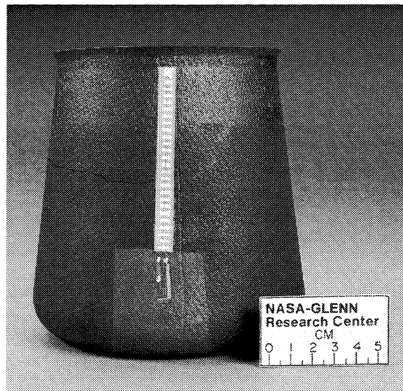
Figure 16 – Condition of a thin film thermocouple on a rich zone liner after combustion exposure.
