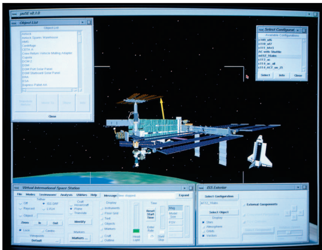
The EZopt program runs a simulation of Space Shuttle docking trajectories.
