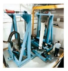
Computed tomography, widely used in the medical field, has proven invaluable to locate imperfections in aerospace components. This Advanced Computed Tomography Inspection System can scan anything from small turbine blades, auto parts, and drums of nuclear waste to rocket assemblies.
