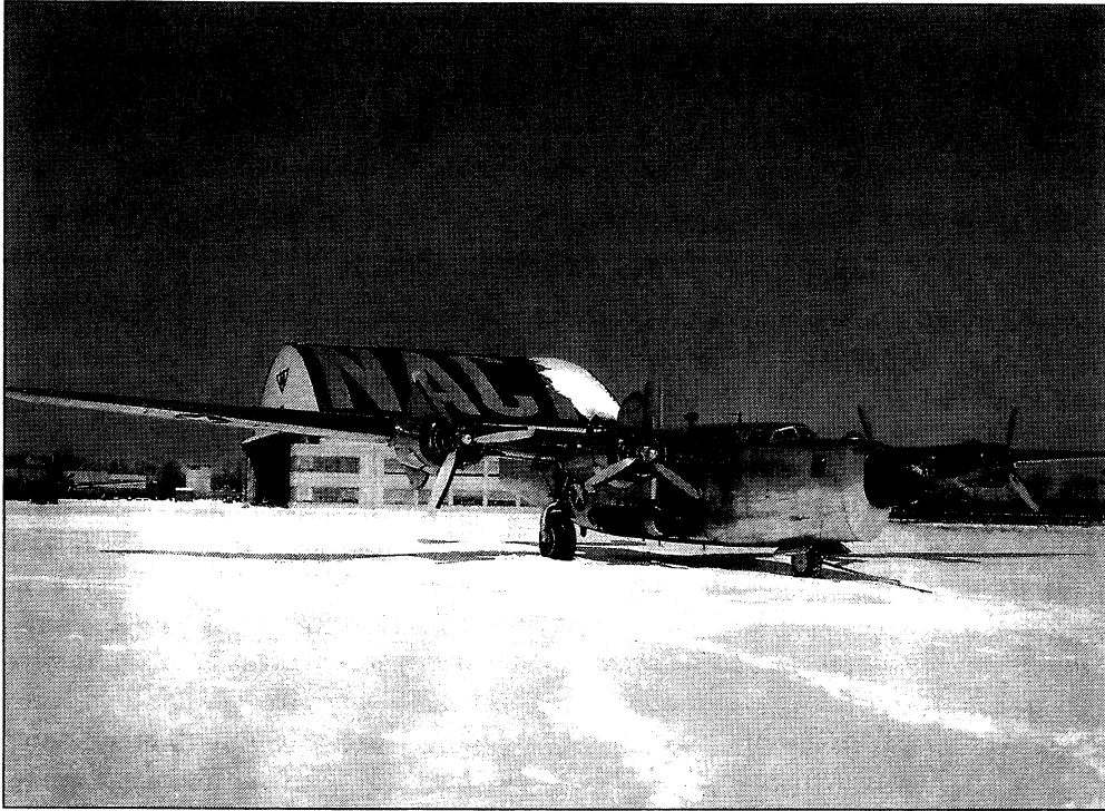
Figure 4-1. B-24 with Westinghouse 24C-2 turbojet engine mounted under wing, 1948. (NACA C-20866)
