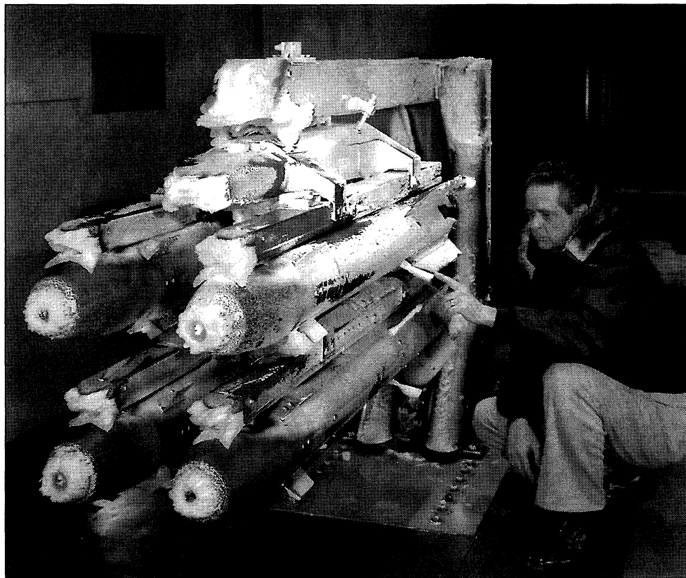
Figure 5-2. Rockwell factory representative inspects Hellfire missiles during IRT test, 1978. (NASA C-78-1039)
