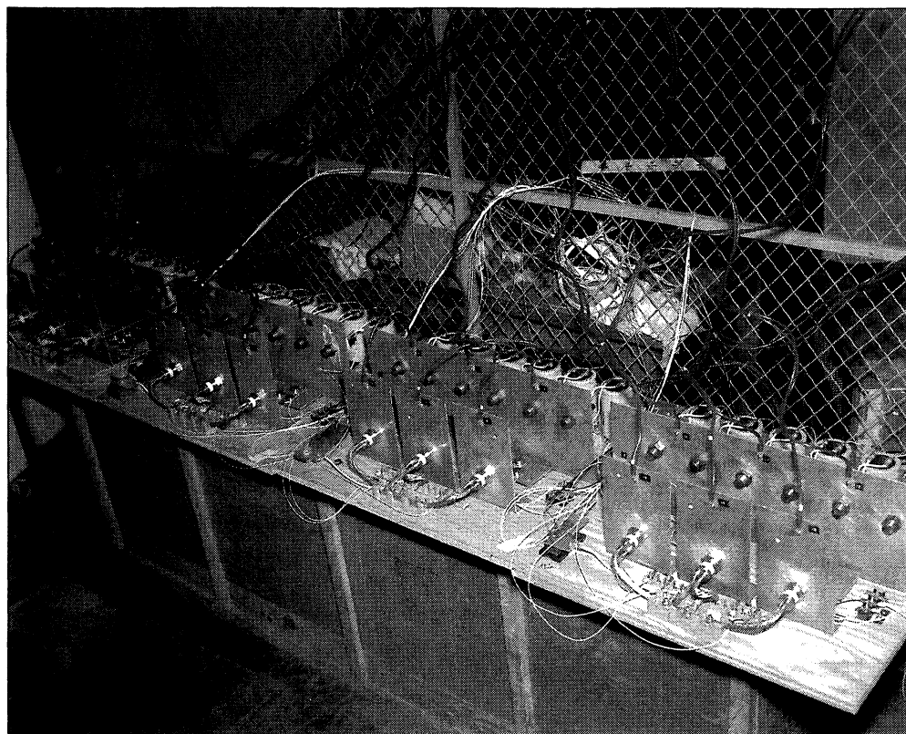
Figure 5-12. Electro-impulse de-icing equipment for McDonnell Douglas tests in the IRT, 1981. (NASA C-81-6007)
