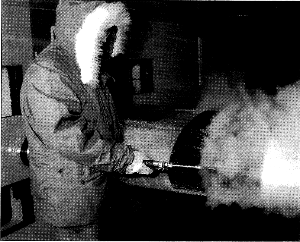
Figure 7-1. William Sexton de-ices model in the IRT, 1992. (NASA C-1992-10571)
