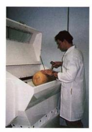
ate socket (bottom opposite) and the prosthetist then modifies, designs and sculpts the socket shape on the computer's monitor. The foam blank is inserted in the computer-directed carver (left below) which carves a positive model. A socket is then "thermoformed" over the model and the patient is ready to be fitted.
