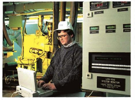
of great concern because of the extensive damage to the machinery caused by jamming; repairs can be very costly and down time/loss of production adds considerably to the cost. The company wanted to know if there was a way to detect the onset of machine jam and automatically shut down the press faster than an operator could to limit or eliminate damage to the machine; avoidance of one serious jam could easily pay for the investment in special monitoring equipment.
