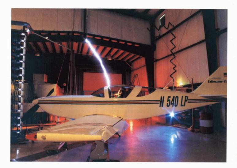
FAA for certification of a factory-produced aircraft. The Glasair III-LP successfully passed this and other tests and became the first kit-built composite aircraft to be lightning tested and protection-verified under the guidelines used by the FAA to certify general aviation aircraft.
