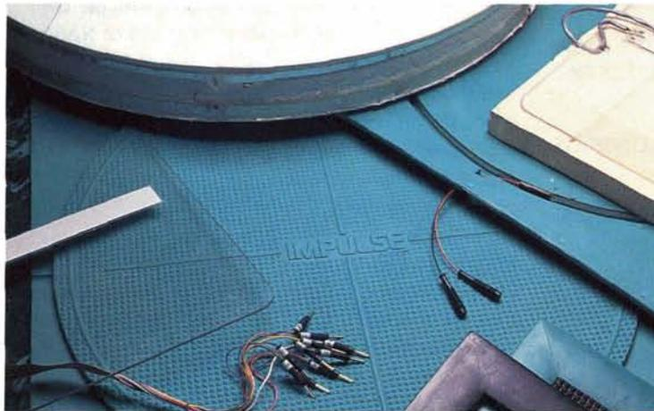
ed to hop in a straight line across a row of platforms on an affected limb; a base line test of the same moves on the unaffected limb provides a comparison. In these photos, the users are working with the smaller of three Biotran models; it has seven sensing platforms in a floor area measuring six by eight feet, along with a 26-inch monitor, a data acquisition
