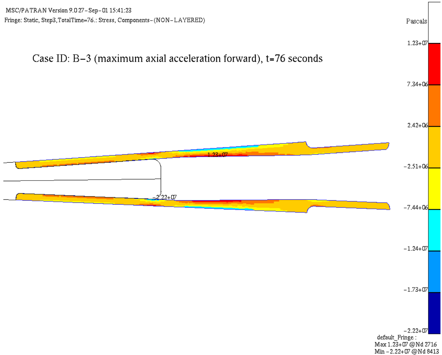
Figure 15: In-plane longitudinal stress ( \sigma_{xx} ) present in the brackets at a time of 76 seconds (corresponding to maximum axial acceleration condition).
